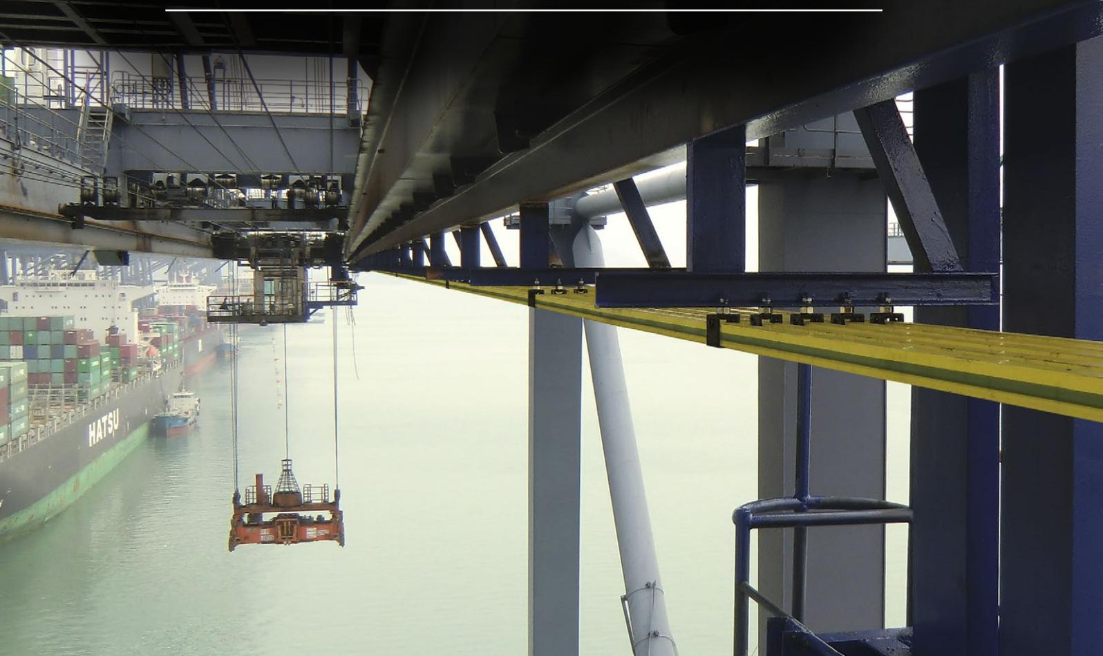
**ProfiDAT®** is the most compact data communication solution on the market. The use of the ground rail for data makes it possible to convert a standard 3+PE (Earth) Conductor Rail configuration into a 3+PE (Earth) data solution – up to 100Mbps – without adding an additional profile. A redundant set of antennas allows the crossing of STS boom hinge points or expansion joints.
