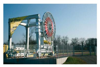
Caption: A nearly authentic and therefore ideal testing area: Testtrack V-Rex on the premises of Wampfler AG in Weil am Rhein with a velocity of up to 300 meters per minute and a traverse path of up to 140 meters. A real load test for motor reels with medium voltage cables.
