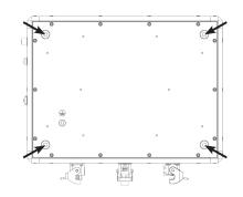
Fig. 7: Fixing holes
