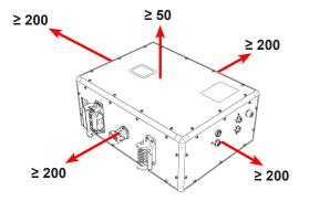
Fig. 4: Clearances around the SCM (mm)
