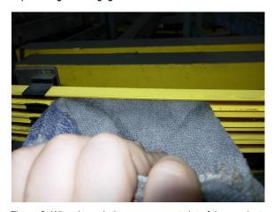
Figure 6: Wipe through the engagement slot of the conductor rail.
